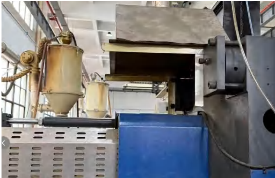
注塑废气集气罩
